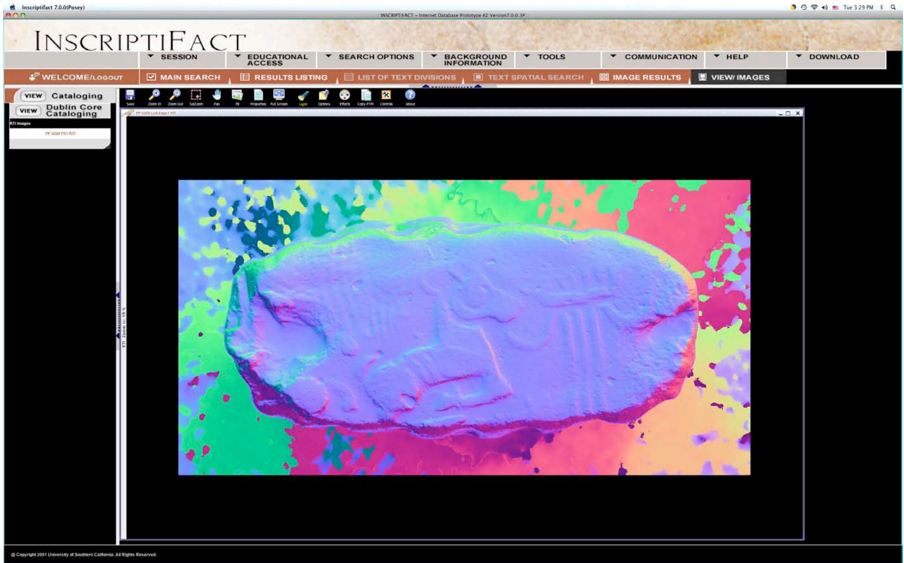
Figure 13: Visualize Normals . Each color represents an angle at which light is being reflected off of the surface of the object, giving one real information about the surface texture.
